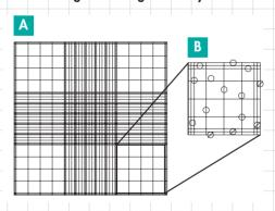
Figure 1 A One chamber of a hemocytometer slide under 10x objective and 10x ocular. The chamber is divided into 9 major squares.
