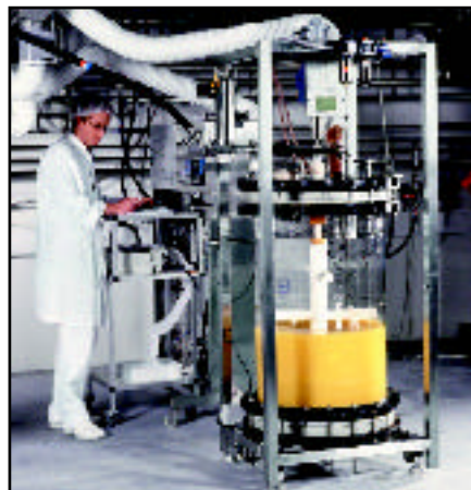
A 270-litre solid phase reactor at PolyPeptide Laboratories A/S (Hillerød, Denmark).
