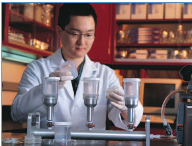
MicroFunnel Plus filter funnels streamline QC testing.
