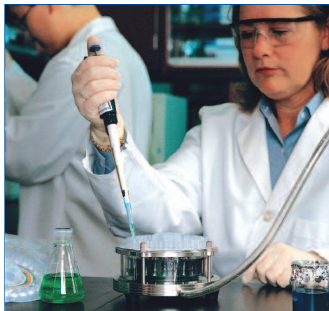
The AcroPrep 24 filtration system simultaneously processes up to 24 samples.
