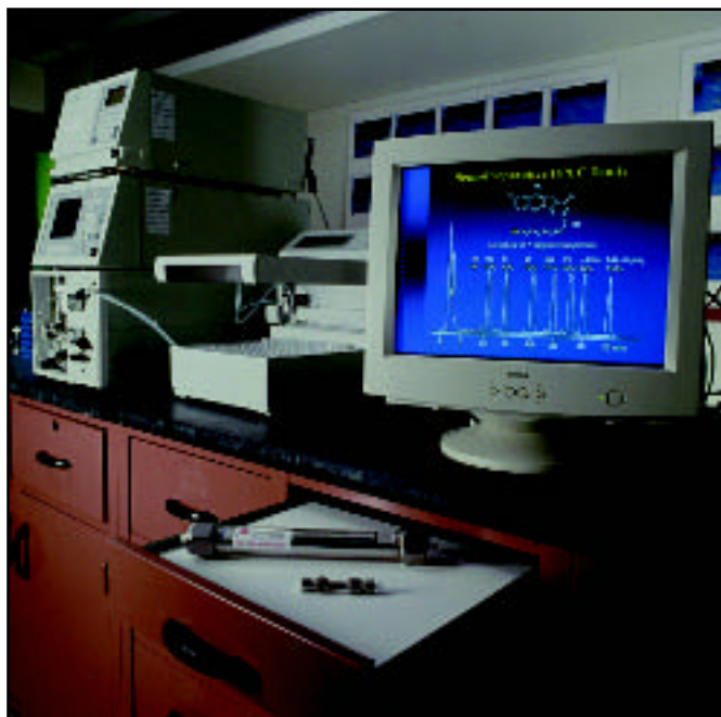
Fluorine HPLC can resolve fluorine-tagged compounds based on fluorine content.
