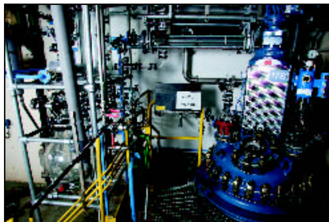
An 800-litre FDA-compliant pilot reactor that forms part of Minakem's fine chemical production facilities.
