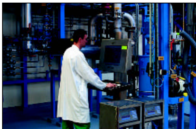
Libragen has established a strategic alliance with fine chemicals manufacturer Minakem. Pictured is Minakem's 600-litre Hastelloy low-temperature reactor, capable of operating down to -100°C.
