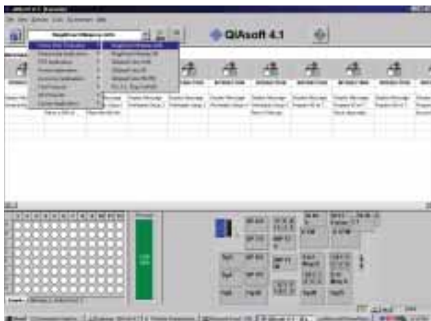
Figure 4 The fully automated MagAttract 96 Miniprep procedure in QIAsoft™, the BioRobot Operating System software. Protocol selection and execution is all at the click of a button, and intuitive user-prompts appear at the start of the procedure.
